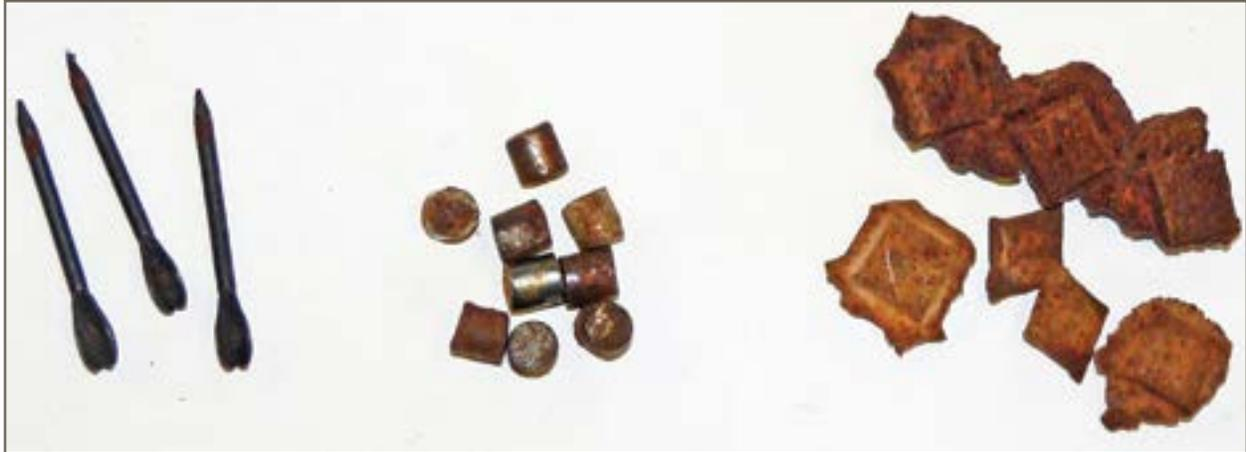
Left to right, the image shows flechettes from a munition, pre-chopped fragments from a bounding fragmentation mine, and pre-scored diamond fragmentation from a submunition.
